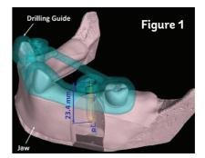
**Figure. 1**: Trial of a dental drilling guide produced by additive manufacturing for the drilling of holes to fit dental implants into artificial jaw models with only few abutment teeth. The drilling angle  $\alpha$  and the drilling depth were measured by means of computed tomography. Source: PTB
