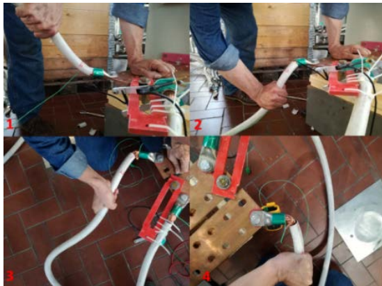
Fig.5. Sequence of the four cable rotations around the lug plane. 1) 45° up, 2) 45° down, 3) 45° to right and 4) 45° to left.
