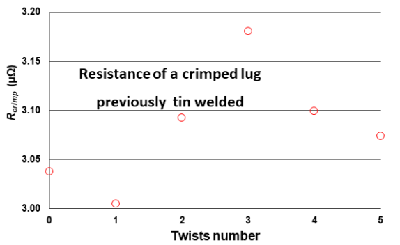
Fig.12. R_{crimp} behaviour of a lug, previously welded and after crimped to a cable undergoing twists.
