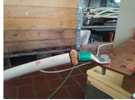
Fig.14. Swelling of the bare cable area.
