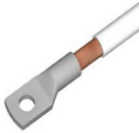
Fig. 1. Lug crimped to a cable.
