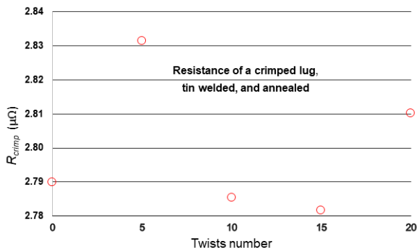
Fig.13. R_{crimp} behaviour of a lug, previously welded, crimped to a cable undergoing twists and annealed.
