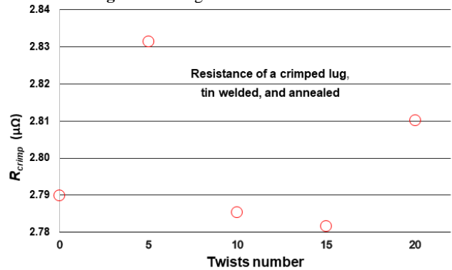
Fig.15. R_{crimp} behaviour of a lug crimped to a cable undergoing rotations on and around the lug plane.
