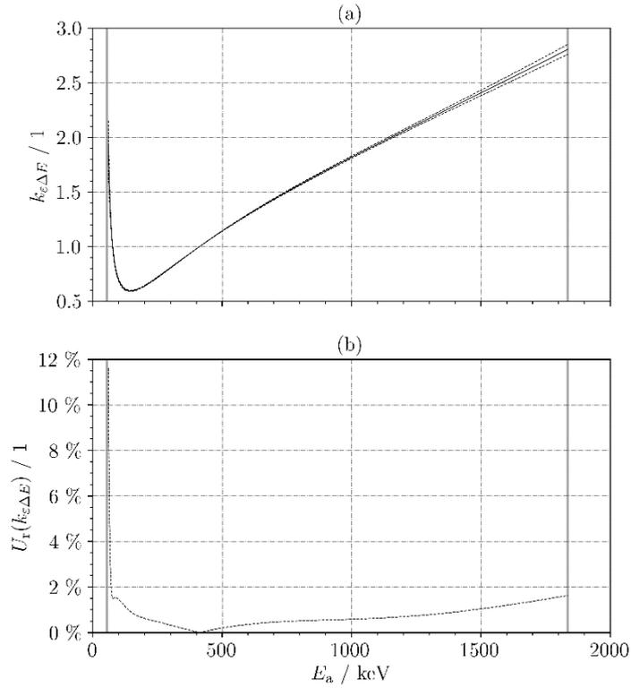
**Figure 5** The  $k_{\epsilon\Delta E}$  function (a) and the corresponding relative expanded ( $k = 2$ ) uncertainty,  $U_r(k_{\epsilon\Delta E})$ , (b) versus  $E_a$  within the range 53.16-1836.07 keV.
