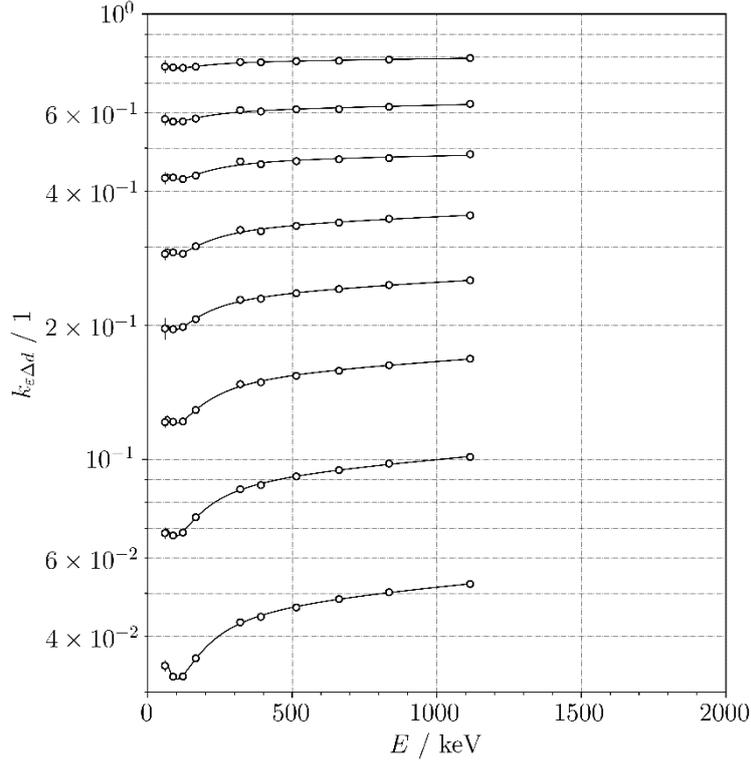
**Figure 3** Fitted  $k_{\epsilon\Delta d}$  functions and  $\frac{\epsilon_{std}(E_r)}{\epsilon_{sm}(E_r)}$  values obtained within the range 59.54-1115.54 keV at the eight sample counting positions with the true-coincidence free  $\gamma$ -emissions of the 12ML01EGMA15 multi- $\gamma$  source. Functions are plotted in vertical descending order from 16 cm to 2 cm distance from the detector end-cap. Vertical error bars, somewhere visible, correspond to the expanded ( $k = 2$ ) uncertainty.
