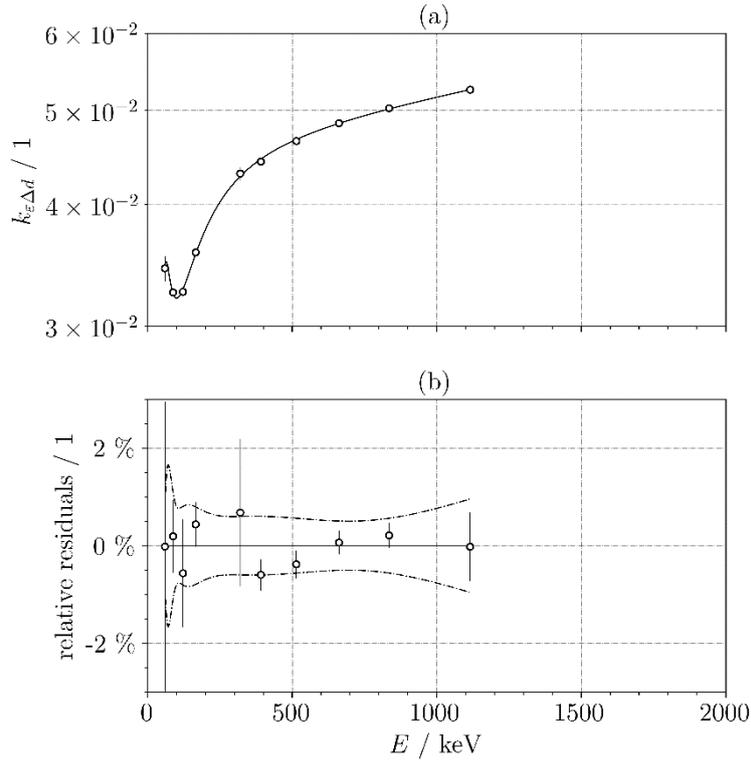
**Figure 4** Fitted  $k_{\epsilon\Delta d}$  function and  $\frac{\epsilon_{\text{std}}(E_r)}{\epsilon_{\text{sm}}(E_r)}$  values within the range 59.54-1115.54 keV at 2 cm distance from the detector end-cap (a), and relative residuals (b). Dashed horizontal lines and vertical error bars correspond to the expanded ( $k = 2$ ) uncertainty of  $k_{\epsilon\Delta d}$  and of  $\frac{\epsilon_{\text{std}}(E_r)}{\epsilon_{\text{sm}}(E_r)}$ , respectively.
