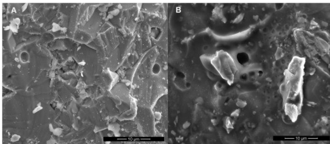
Fig. 8. SEM images of the surface of coarse particles ( $\sim 1$  mm) of the  $\text{La}(\text{Fe,Si,Mn})_{13}$  compound: A) dehydrogenated compound before the sonochemical treatment; B) sonochemically treated sample with the characteristic traces of microcavities induced by bubbles formation/collapse.
