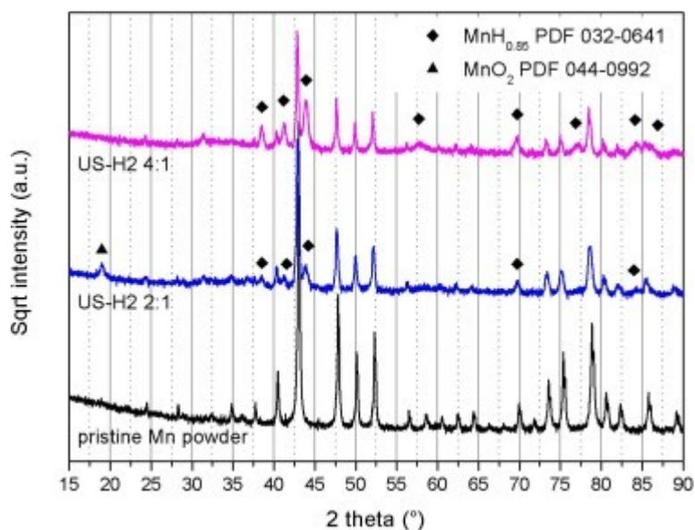
Fig. 3. X-ray diffraction patterns of selected Mn samples treated in  $\text{NaBH}_4$  solution. Symbols identify the phases corresponding to the Powder Diffraction File (PDF) quoted in the legend. Peaks without symbols correspond to  $\alpha\text{-Mn(H)}$ .
