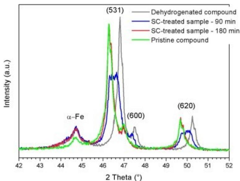
Fig. 6. X-ray diffraction patterns of the La(Fe,Si,Mn)<sub>13</sub> samples, before (dehydrogenated compound) and after (SC-treated samples) sonochemical treatments of different duration. The XRD pattern of the pristine compound (the starting powder prior to hydrogen desorption by thermal annealing) is also reported for comparison. A small angular range is considered to better display the peaks shift. Indexed peaks correspond to the cubic La(Fe,Si,Mn)<sub>13</sub>(H) phase.
