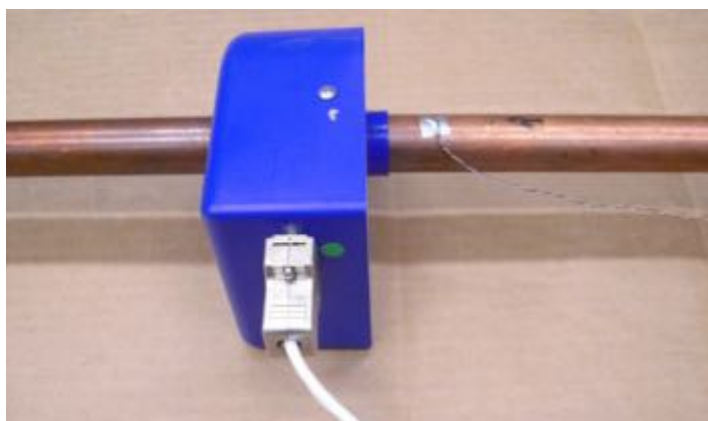
Figure 2. Bus-bar rod and temperature measurement of the rod.
