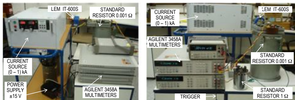
Fig. 2. Workplace for LEM IT – 600S calibration
