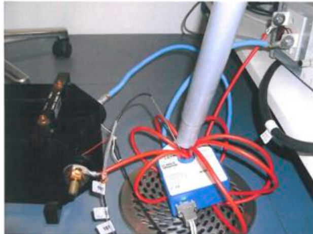
Figure L1: Some details of one of the measurement setups. On the left the 10 mΩ resistor, the voltage measurement wires going to the DMM are also visible. In the middle the travelling ZFCT with 8 loops of cable around it, the temperature sensor measuring on the surface of the cable from inside the ZFCT, a vacuum cleaner pipe coming from up. On the right the HP 100 A current source.
