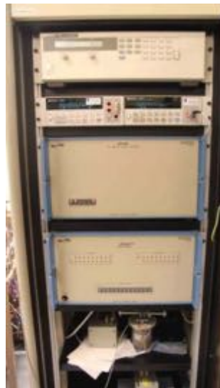
Figure 1. Measurement rack with the low-ohmic resistance bridge which consists of (from top to bottom): a HP6672A DC current source, a HP34401 current meter, a HP34420A null detector, a MI-6011A range extender, and a MI-4220A low thermal matrix scanner. Below the matrix scanner two reference resistance standards can be seen.
