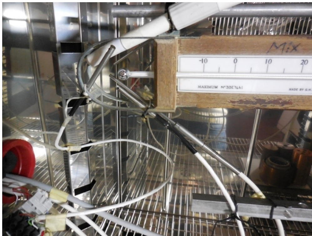
Figure 5. Close up view of the sensing element, mercury bulb and INRiM four Pt 100 reference thermometer. The four Pt 100 are not in contact with any of the two thermometer to avoid self-heating to be transferred to the devices under test.
