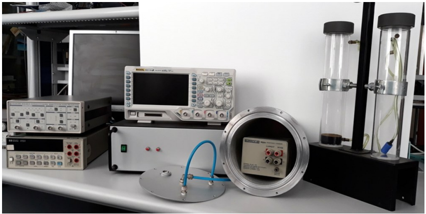
Fig. 2 - Setup for standards characterization vs. pressure and humidity.
