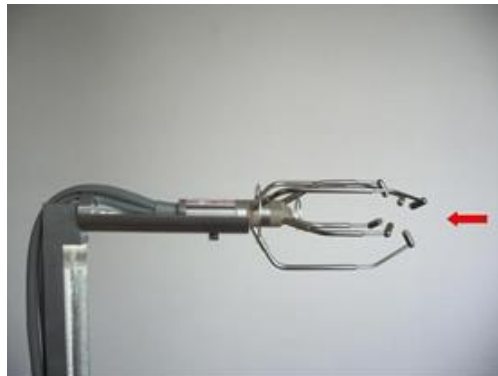
Fig.1. Ultrasonic Anemometer sensing element (the arrow indicates the flow direction)
