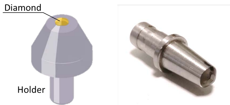
Fig. 1. 3-D model (left) and picture (right) of a typical Vickers indenter.
