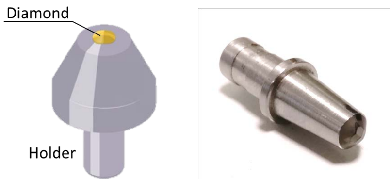
68 Fig. 1. 3-D model (left) and picture (right) of a typical Vickers indenter.
