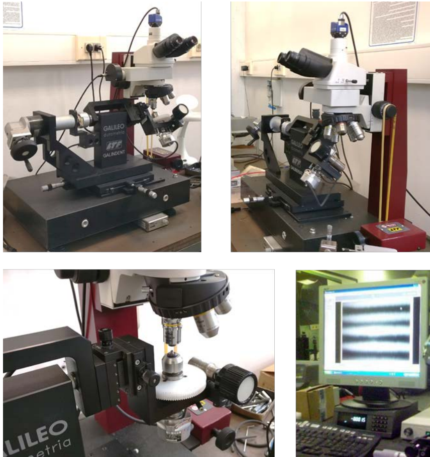
Fig. 3. The Galileo-LTF® Gal-Indent optical system used at INRiM hardness laboratory for the measurement of the vertex angles and the quadrilateral base angles.
