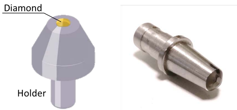
68 Fig. 1. 3-D model (left) and picture (right) of a typical Vickers indenter.
