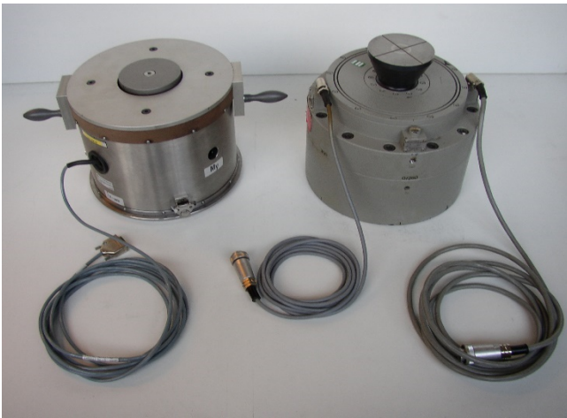
Figure 2: Photograph of the two 1 MN force transducers
