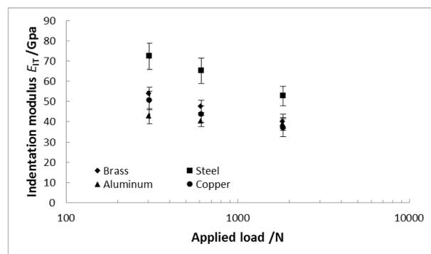
Figure 14: Indentation modulus calculated using the Brinell method ( $R=1.25$  mm).
