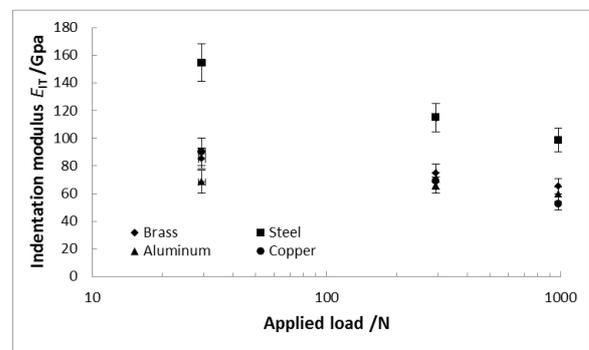
Figure 12: Indentation modulus calculated using the Vickers method.
