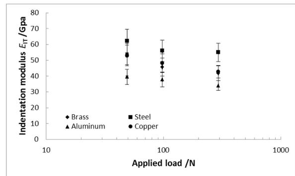
Figure 13: Indentation modulus from Brinell method ( $R=0.5$  mm).
