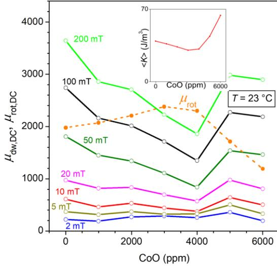
Fig. 1. Rotational (dashed line)  $\mu_{rot,DC}$  and dw  $\mu_{dw,DC}$  dc permeabilities versus CoO content.  $\mu_{rot,DC}$  is obtained according to the decomposition method discussed in [Beatrice 2017]. Magnetic softening occurring at intermediate CoO values is associated with an increased role of the rotations with respect to the dw displacements. The inset shows the correspondingly calculated behavior of the effective average anisotropy  $\langle K \rangle$ .
