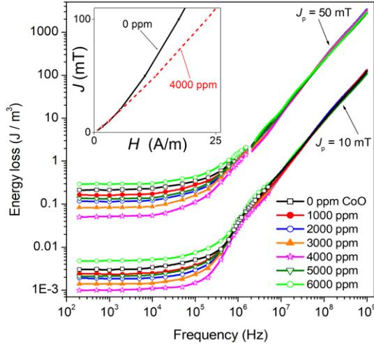
Fig. 3. Energy loss versus frequency at  $J_p = 10$  mT and  $J_p = 50$  mT up to CoO = 6000 ppm. Symbols and continuous lines refer to fluxmetric and VNA measurements, respectively. The 4000 ppm CoO sample exhibits the lowest loss figure up to a few MHz, where all curves tend to coalesce. Inset: normal  $(J, H)$  dc curves within the Rayleigh region for CoO = 0 and CoO = 4000 ppm.
