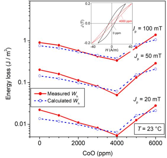
Fig. 2. Quasi-static energy loss  $W_h(J_p)$  measured versus the CoO content at three different  $J_p$  values and its prediction using (4). The dc hysteresis loops shown in the inset put in evidence that softening by CoO addition takes place by simultaneous decrease of coercive field and irreversible permeability.
