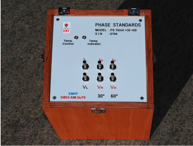
Figure 7. Schematic (a) of the positive phase standards and photograph (b) of the 0104 standard. As for the negative standards, the box in figure (b) contains two phase standards, which are identified in this work with the suffixes “A” (left) and “B” (right). The sockets labelled Temp. Control and Temp. Indicator are connected to two thermistors sensing the box temperature, one for the external temperature controller and one for the operator.
