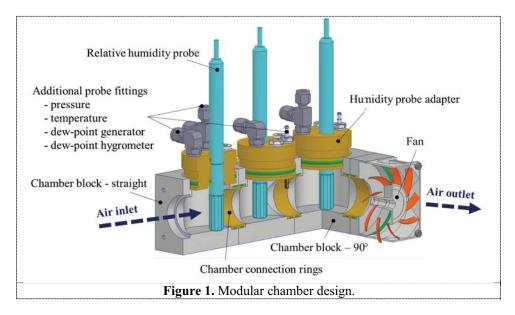
While the assembly presented in Fig. 1 is appropriate for supplying with the air prepared in the climatic chamber, it can also be supplied from DPG. For this purpose, a fan should be removed, and
