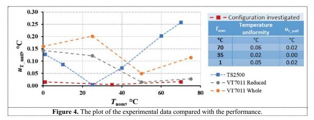
When expressed as RH at the nominal temperatures, the uncertainty due to temperature uniformity always corresponds to a value lower or equal to 0.06 %rh at a nominal RH of 50 %rh. The temporal stability of the air temperature monitored during 30 min was always lower than 5 mK.
