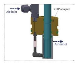
**Figure 2.** Additional miniature sub-chamber for reducing the RHPs self-heating effects when using the DPG as the gas supply. Air exits to the chamber volume and then flows out the chamber through one of the adapter bores.
