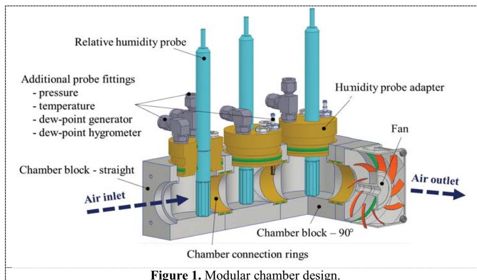
**Figure 1.** Modular chamber design.
