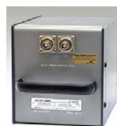
Fig. 5. 1 nF ESI SC1000 standard capacitor.
