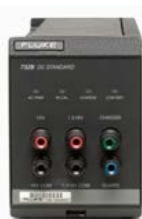
Fig.1. J. Fluke mod. 732 B DC Voltage standard.
