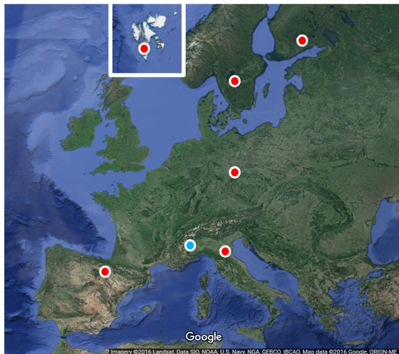
Figure 2. A map of the stations involved in the IVS EUR137 experiment. Red circles indicate the VLBI radio antennas; in blue, the position of the Italian National Metrology Institute. (Imagery ©2016 Landsat, Data SIO, NOAA, U.S. Navy, NGA, GEBCO, IBCAO, Map data ©2016 Google, ORION-ME)
