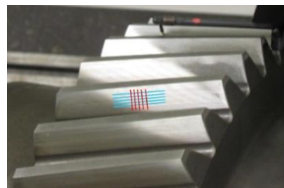
Figure 1. Scan paths along the gear tooth: involute direction (red); helix direction (blue).
