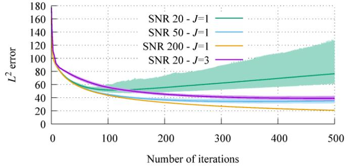
Fig. 2. Trend of the median (solid lines) and shortest 95 % coverage interval (bands) of the  $L^2$  norm of the error in  $\chi$  against the number of iterations of CSI-EPT for different SNR and coil settings. The 16 legs birdcage is considered.
