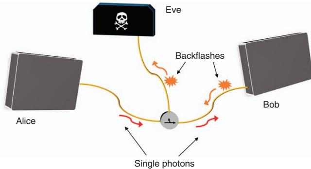
**Figure 1** Representation of an eavesdropper attack exploiting backflash light. Alice sends the photons of the key to Bob; when the photons are detected by Bob using a SPAD, a flash of light, the backflash, is emitted back to the channel. Eve can use a circulator to intercept this spot of light to acquire information about the detector that has clicked.
