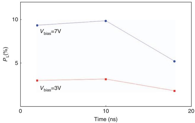
**Figure 5** Information leakage as a function of the arrival time of laser photons with respect to the gate window that triggers the DUT. The data were collected for DUT1 operating at different bias voltages of 7 and 3 V.
