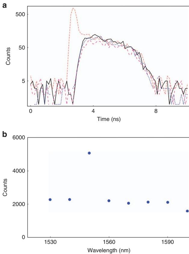
**Figure 6** (a) Temporal distributions of the backflash counts after spectral filtering, with the filter centered at 1530, 1550, 1570 and 1600 nm. (b) Total counts of backflash light in the observed spectral range (from 1530 to 1600 nm). All measurements were performed using filters with a 10-nm bandwidth.
