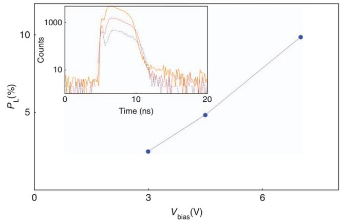
**Figure 4** Information leakage  $P_L$  as a function of the excess bias voltage for the prototype detector DUT1. The peaks of the back-reflected light is presented in the inset (the continuous, dashed and dot-dashed lines represent the cases of 7, 4.5 and 3 V, respectively); the smaller peak due to the reflection of the laser light from the diode surface is relatively more evident at low excess bias voltages.
