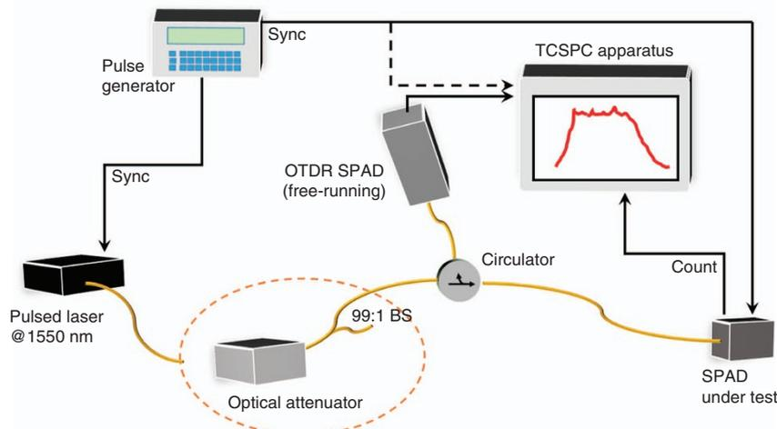
**Figure 2** A schematic representation of our experimental setup. A photon-counting OTDR observes backflash light from the SPAD under test. The source is an attenuated pulsed laser emitting at 1550 nm. The backflash light is detected by a free-running InGaAs/InP detector. Time stamping of detected light is obtained by means of a time-correlated single-photon counting (TCSPC) apparatus.
