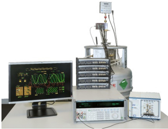
Figure 2. AC quantum voltmeter used to calibrate a calibrator, after reference [45].
