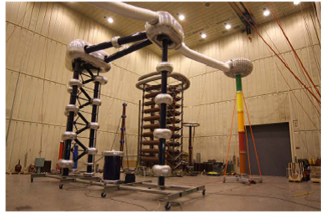
Figure 3. The modular 1000kV divider in a high voltage laboratory. Left, HVDC source and its divider; right, multicolour modular divider.
