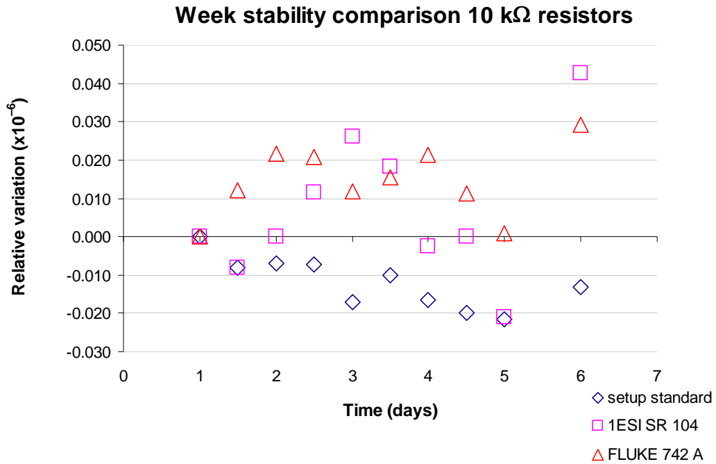
Fig. 10. Week drift of the 10 kΩ setup standard in comparison with two metrology-grade 10 kΩ standards.
