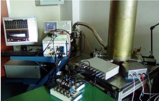
Fig. 2. Photo of the experimental setup based on a reconfigurable electronics for direct synthesis of current-bias setpoints of PJVS SNIS chip and high precision sampler (on the left) and a 3.6 K two-stage cryocooler system (on the right).
