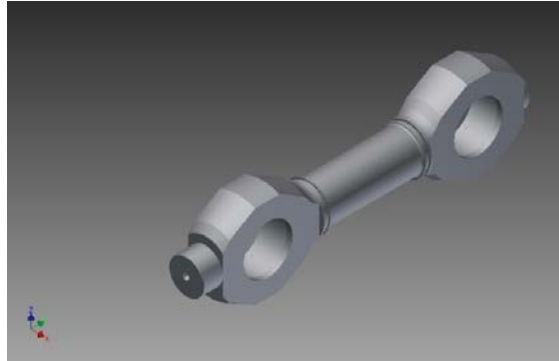
Fig. 1 Structure of the uniaxial force transducer (UFT)
