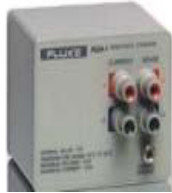
Fig. 2. Fluke 742A 1 \Omega standard resistor.
