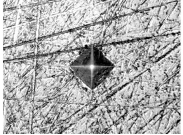
Figure 1: Microscopic image of a typical Diamond Pyramid Hardness (DPH) impression from a Vickers hardness test on a metallic surface.
