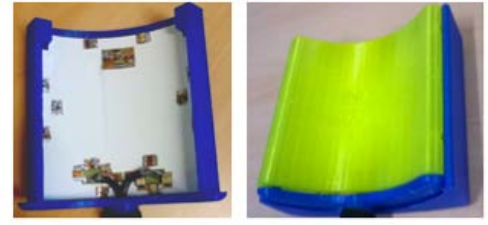
Fig.3: Double-tuned 1H/23Na planar antenna polylactide (PLA) thermoplastic mechanic support
