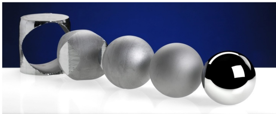
Figure 4. Steps for manufacturing nearly perfect silicon spheres.
