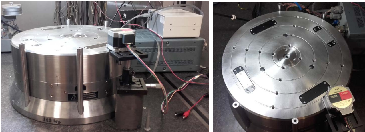
Figure 3. Picture of the REAC: side view on the left; top view on the right. The four windows visible on the top are the access to the four reading heads of the two encoders.
