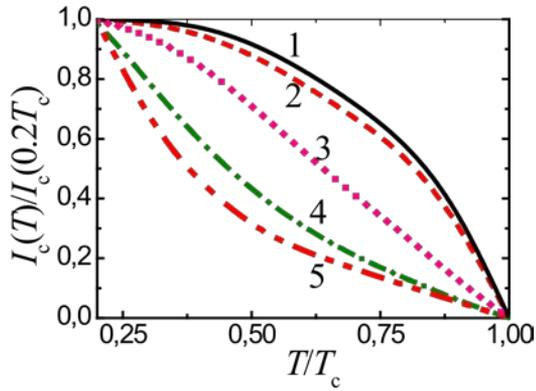
Fig. 1.  $I_c$ -vs- $T$  curve simulations for a standard SIS junction [15] (curve 1); an S/N-I-S device with a non-superconducting and thick ( $d_{Al} = 120$  nm) Al interlayer and an I barrier with the transparency  $D_I = 0.1$ , the model *b* (curve 2), and S/N-I-S heterostructures with a non-zero superconducting order parameter in the Al interlayer, the model *a* ( $d_{Al} = 60, 120, 200$  nm for curves 3, 4, and 5, respectively).
