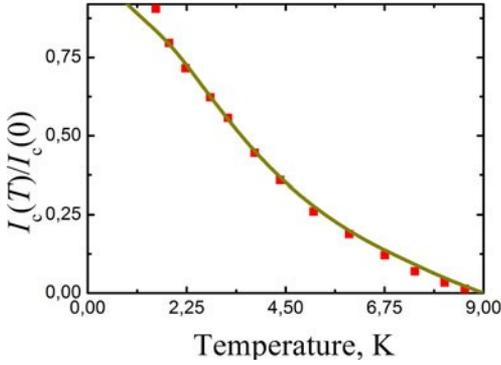
Fig. 2. Representative  $I_c$ -vs- $T$  dependence for Nb/Al-Al oxide-Nb junctions with thick Al interlayers and ultra-thin Al-oxide barriers. Experimental data and results of numerical calculations within the model *a* are shown by squares and a solid line, respectively. In both cases the thickness  $d_{\text{Al}} = 120$  nm.
