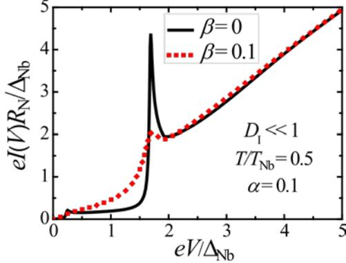
Fig. 3. Dissipative current-voltage characteristics of an S/N-I-S junction calculated within the model *b* in the tunneling regime ( $D_1 \ll 1$ ),  $R_N$  is its resistance in a normal state; the two curves show an effect of the electron mean free path in the N interlayer.
