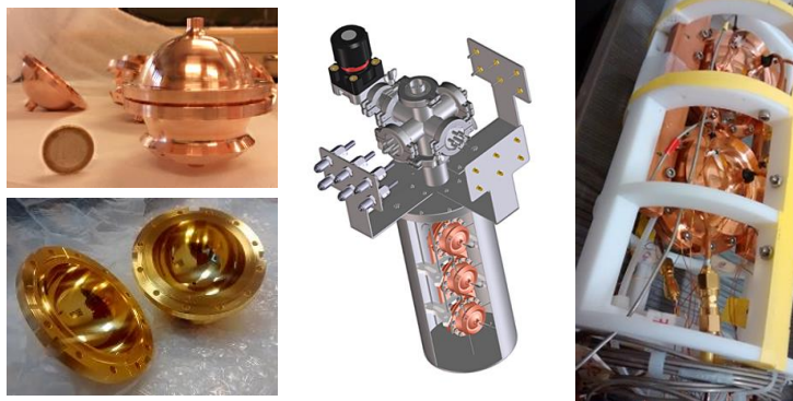
Figure 4: second generation of microwave hygrometers and their assembly
