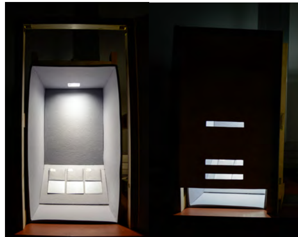
Figure 2 Observation box with samples on the exhibition plane left, with the observation shield right.
