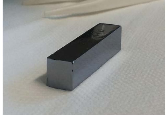
Figure 1. The Si sample after the deep etching following the annealing at 740 °C and slow cooling.
