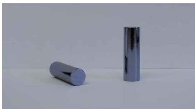
Figure 1. The two samples of the ^{28}\text{Si} -enriched cut from the AVO28 crystal.
