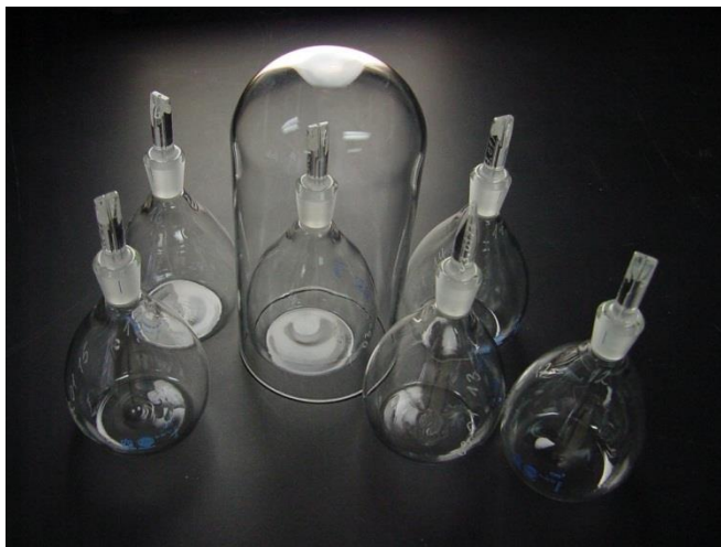
Fig. 2. Image of the 100 mL transfer standards
