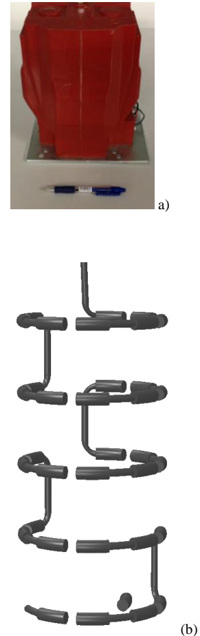
Fig.7. Structure of the 20 kV VD. a) sealed with insulation; b) the FEM model (here without insulation).
