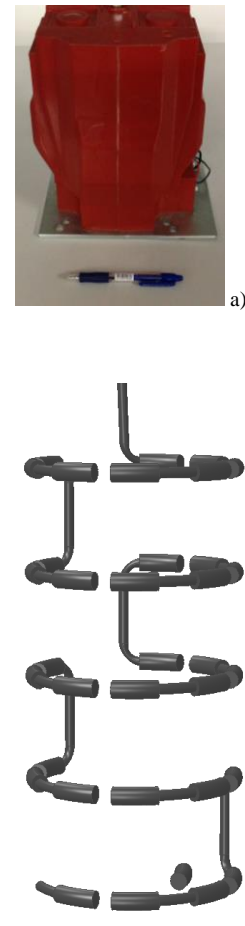
Fig.7. Structure of the 20 kV VD. a) sealed with insulation; b) the FEM model (here without insulation).
