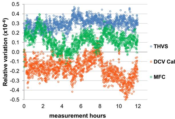
**Figure 3.** 12h spread and drift comparison among the THVS, a DCV Calibrator and a MFC at 100 V reading with a high accuracy DMM.
