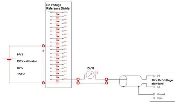
Figure 7. Measurement setup to calibrate the THVS.
