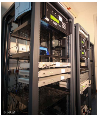
Fig. 8. Picture of the devices realizing the UTC(IT), Exp TA(IT), and UTC(IT) back up time scales steering algorithms
