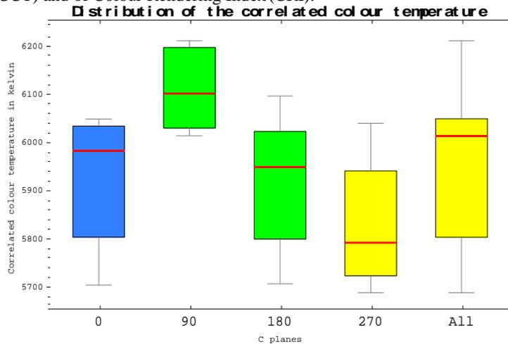
Figure 1 Spatial distribution of CCT of a LED luminaire, in the 4 main C planes (Spatial reference system CIE C<sub>γ</sub>)
