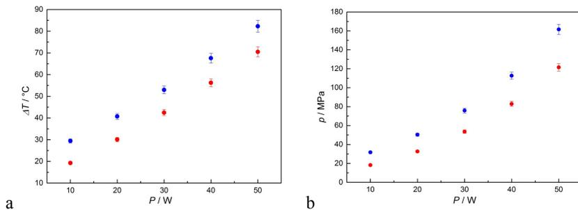
Fig. 3. (a) Temperature rise,  $\Delta T$ , as a function of ultrasound beam power,  $P$ : ● TMM 1, ● TMM 2; (b) Acoustic pressure,  $p$ , as a function of ultrasound beam power,  $P$ : ● TMM 1, ● TMM 2.
