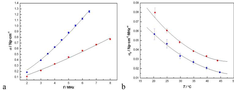
Fig. 2. (a) Attenuation,  $\alpha$ , values and respective uncertainty as a function of the frequency,  $f$ , at  $T = (20.3 \pm 0.7) ^{\circ}\text{C}$ : ● TMM 1, ● TMM 2, - fitting curve; (b) Attenuation coefficient,  $\alpha_0$ , values and respective uncertainty as a function of the temperature,  $T$ : ● TMM 1, ● TMM 2, - fitting curve.
