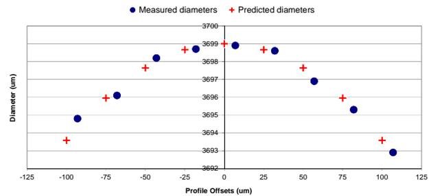
Figure 3. Diameter measurements (solid circle) from nine parallel traces at  $25 \mu\text{m}$  increments through the central region of the Brinell indentation. Also shown are predicted diameter values (cross) based on a circular indentation.
