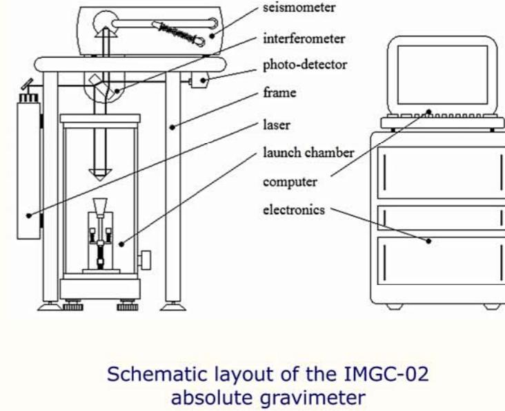
Picture of the new absolute gravimeter IMGC-02
