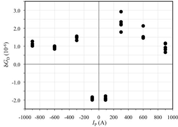
Figure 4: The relative gain error  $\delta G_D$  of the DCCT under calibration, for different nominal primary current values  $I_p^{(n)}$ . Each dot corresponds to half of the measurement cycle shown in Fig. 3. For each  $I_p^{(n)}$ , five measurement results are reported. The average value and its uncertainty are given in Tab. 1.
