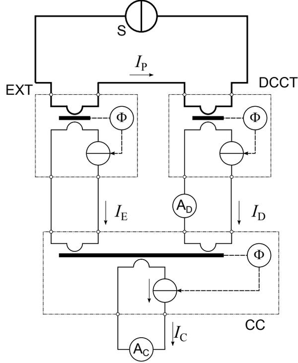
Figure 1: Principle schematics of the DCCT calibration setup.  $S$  is the high-current source,  $EXT$  is an automated current range extender,  $CC$  a dc current comparator. Meter  $A_D$  monitors the DCCT output  $I_D$ ; meter  $A_C$  give the reading of  $I_C$  employed in the measurement model Eq. (2).
