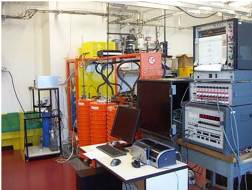
Figure 11. Typical design of a GCHP developed at LNE-Cnam [34, 35].
