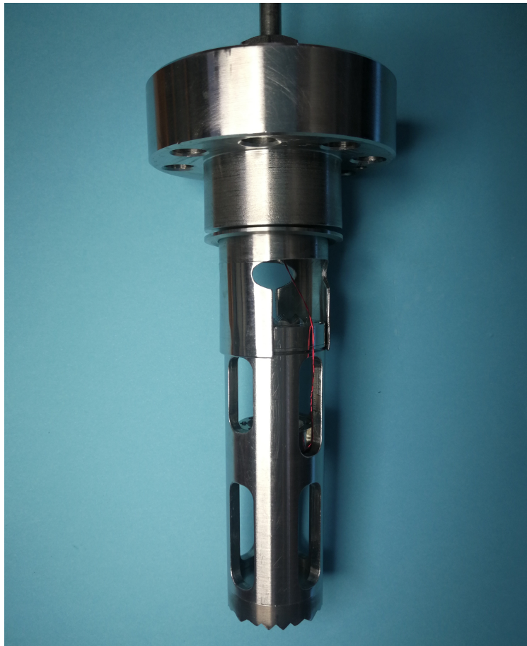
Figure 3: Ultrasonic cell and vessel stopper with coupling holders.
