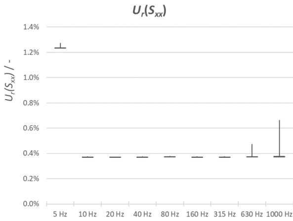
Fig. 6. Relative expanded uncertainties of the 100 MEMS  $x$ -axis sensitivities as function of frequency.
