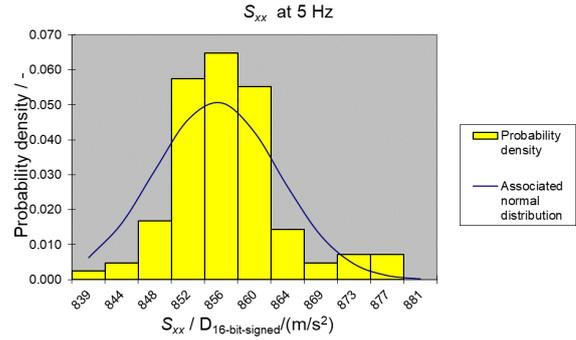
Fig. 9. Distribution of the 100 MEMS  $x$ -axis sensitivities at 5 Hz.
