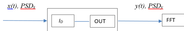
Fig. 4. Setup to evaluate the noises at the detector whose output circuit is connected to a FFT analyser.
