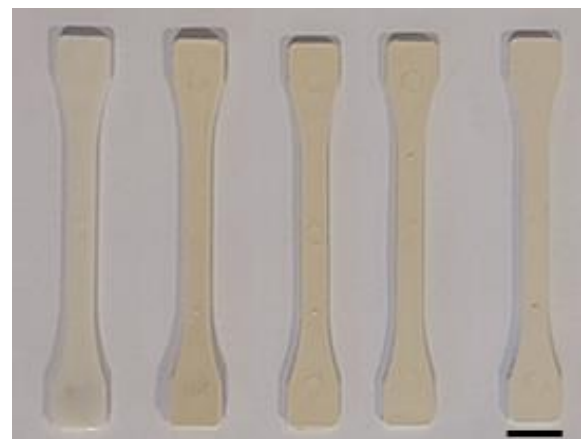
Figure 2. Injection-molded specimens at different ZTC content: from left to right the ZTC wt% varies from 0 to 40% (the dimensional marker is equal to 1 cm).
