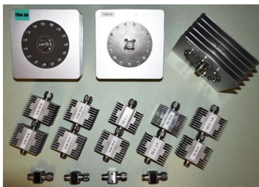
Fig. 4. Set of coaxial shunts built at INRIM and employed for primary alternating current scale realization and as phase standard for currents from 20 mA up to 7 A and frequencies up to 100 kHz.
