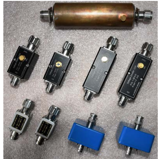
Fig. 3. New set of wideband coaxial resistive dividers for voltages ranging from 1 V to 150 V and frequencies up to 1 MHz. Construction details of 1:52 ratio RVD are given in [7].
